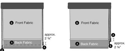
There will be a difference of approx.  $2 \frac{3}{4}$  " between the chain / cord loop that activates the back fabric (A) and the chain / cord loop that activates the front fabric (B).
